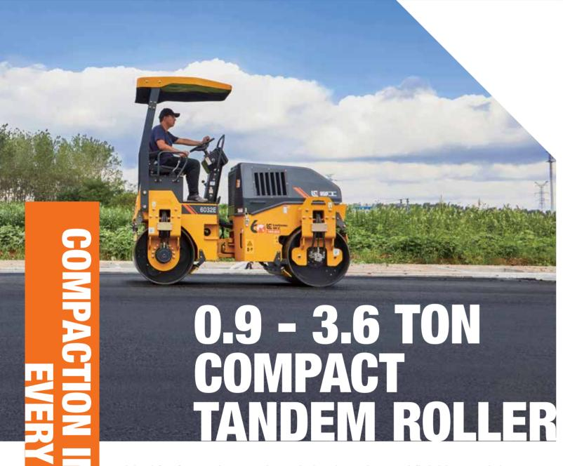
Ideal for footpaths, repair work, landscaping and finishing work in road construction, our compact rollers are highly versatile.
