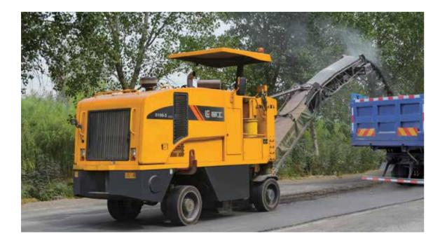
Our 5100-2 milling machine uses high pressure rotary milling technology, utilizing a Hydrostatic drive milling drum with Overloading protect function to greatly increase production efficiency.
